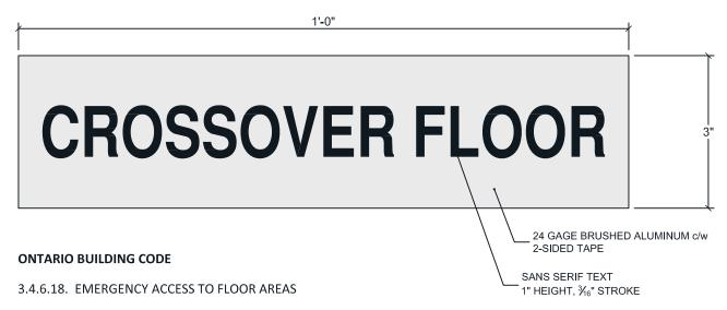
The Building Code requires that in a building over 6 storeys, emergency access is required to be provided out of an exit stairwell to permit people to leave the stairwell and enter a floor area, should the stairwell become blocked by smoke or other obstructions above the exit level. Signs are required to indicate which doors within the exit stairs will provide emergency access to the floor areas.
